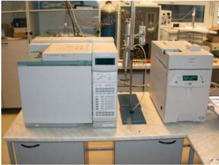
Gas chromatographs (left) and incubation box with glass bottles with soil samples (right).
