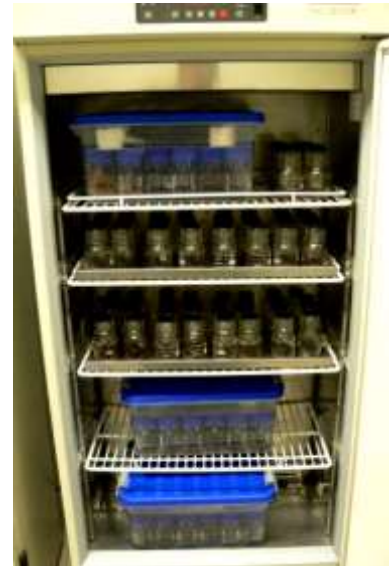
Gas chromatographs (left) and incubation box with glass bottles with soil samples (right).
