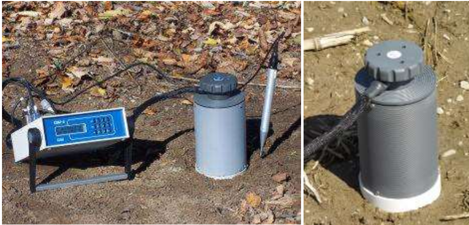
Soil respiration measurement in the field using EGM4 with soil respiration chamber.
