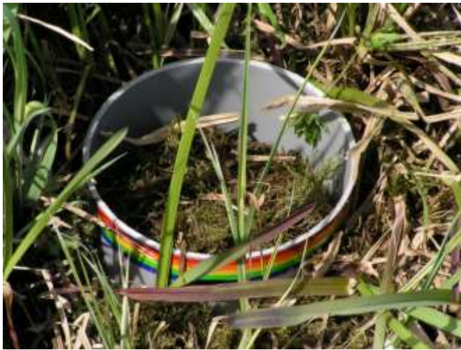
Plastic collar inserted into the soil for soil respiration measurement.
