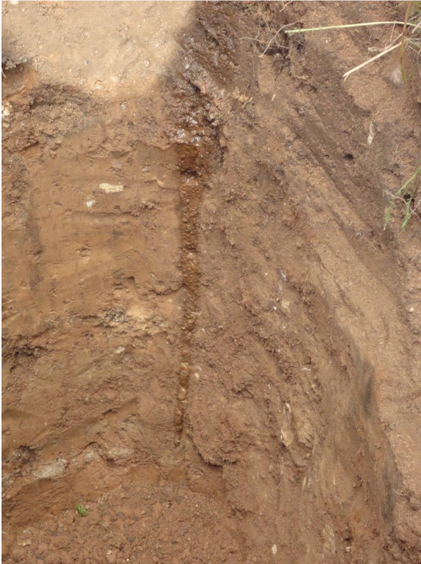
Figure 2 : “Boiling”-test by tipping HCl solution down the several horizons
