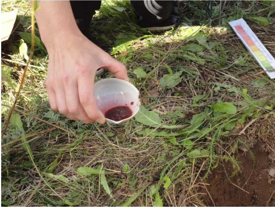
Figure 3: Showing the color change range of universal indicator. As soil itself was alkaline, the acid was added to the dish to get red reaction.
