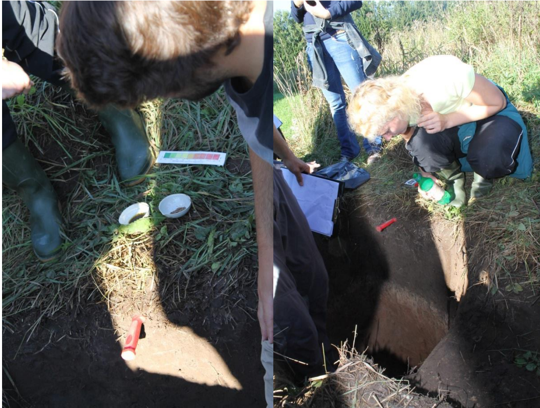
Figure 9: pH measurement with universal indicator. Figure 10: HCl test for lime content.
