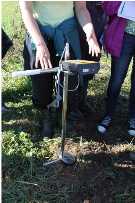
Figure 12: Percometer used to measure the soil water content and salt content.
