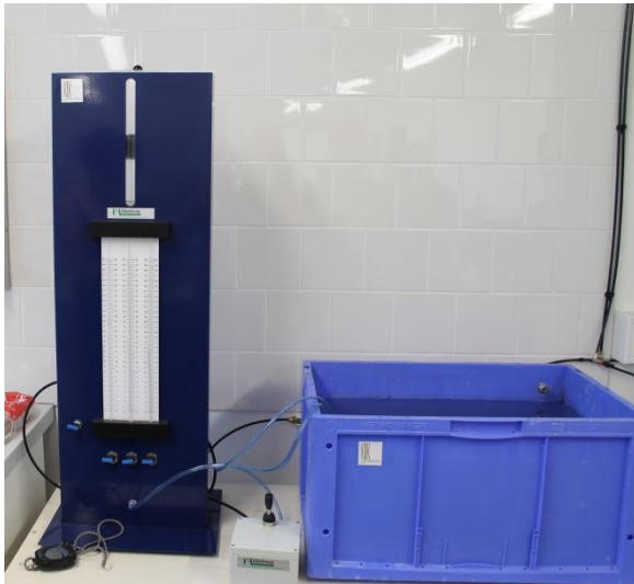
Figure 4: Device to measure the soil permeability.
