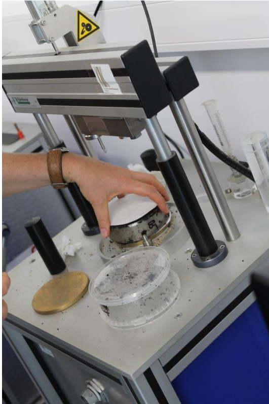
Figure 2: Device to measure the soil compaction.
