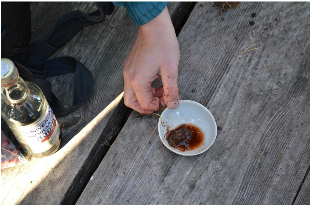
Fig. 1: Testing the pH value with universal indicator.
