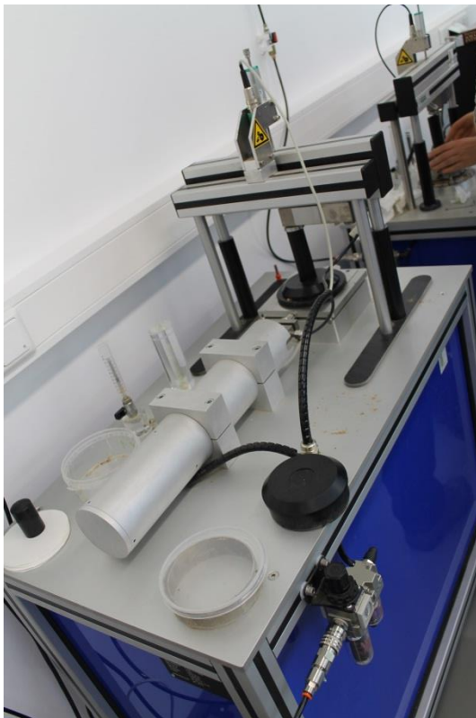
Figure 1: Device to measure the shear strength.
