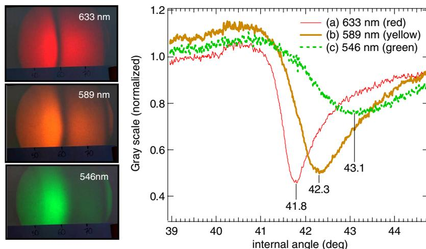
**Figure 7.** The plasmon profile obtained with different wavelengths. The three photos of the left panel show the reflected beam exhibiting a black stripe due to the plasmon extinction. The light source is a white light filtered with narrow-band interferential filters. The plasmon shifts from  $41.8^\circ$  up to  $43.1^\circ$  as the wavelength decreases. The most striking effect is the damping of the SPR due to the coupling with the interband transitions of gold.
