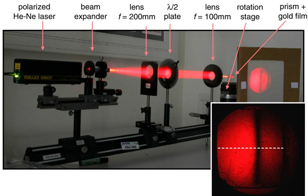
**Figure 6.** Optical setup for directly measuring the plasmon extinction. A digital photograph of the divergent beam reflected by the gold thin film is shown and the intensity of light is digitized along the dashed line. The profile is normalized to the intensity profile obtained with  $s$ -polarization. The resulting plasmon curve is given in figure 5(b).
