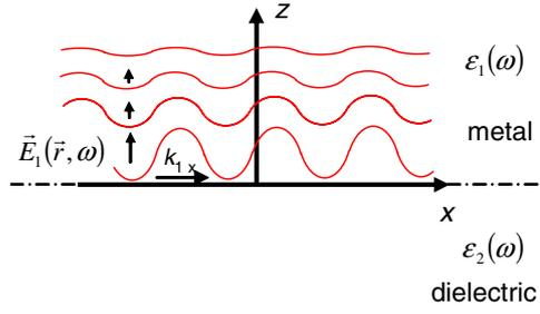
**Figure 1.** Structure of a surface wave (evanescent wave). The wave propagates along the  $x$  direction with a wavevector  $k_{1x}$  and has an exponentially vanishing amplitude in the direction normal to the interface (direction  $z$ ). In the  $z$  direction the decay length is given by  $1/k_z$  and there is no propagation but an oscillation of the electric field as a whole.
