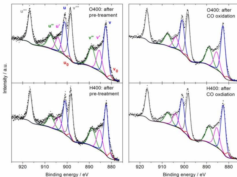
**Figure S1.** XP spectra of the Ce(3d) region of a 4.5wt.% Au/CeO<sub>2</sub> catalyst recorded *ex situ* after O400 (top) and H400 pretreatment (bottom). Left panels: before, right panels after CO oxidation reaction (1000 min, 1% CO, 1% O<sub>2</sub>, rest N<sub>2</sub> at 80°C).
