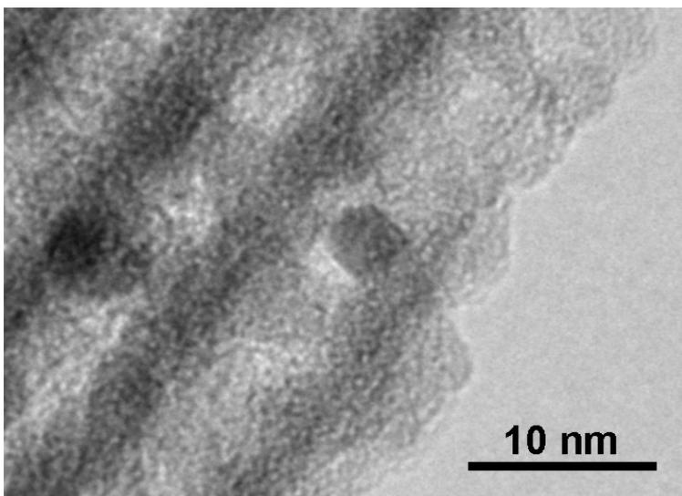
Fig. 2: HRTEM micrograph of a Au particle in mesoporous  $\text{SiO}_2$ . From interface analysis it can be concluded that this particle is located inside of the pore.
