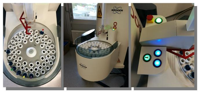
Sample Case Plus autosamplers will be used on all new NMR-spectrometers. Button usage for manual autosampler control should be **avoided**.
