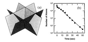
FIG. 16. Inverted-pyramid trap used for Raman cooling. (a) Schematic of the trap geometry, and (b) lifetime measurement performed after Raman cooling at a background pressure of  $\sim 3 \times 10^{-11}$  mbar. From Lee et al. (1996).
