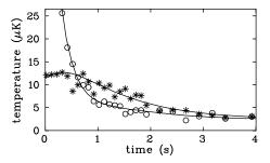
FIG. 21. Cooling dynamics in the GOST. The vertical  $(\circ)$  and horizontal  $(\bullet)$  temperatures measured for about  $10^5$  trapped Cs atoms are plotted as a function of the storage time. The solid lines are theoretical fits based on Eq. 52 and the assumption of an EW reflection with a small diffusive, non-specular component. From Ovchinnikov et al. (1997).
