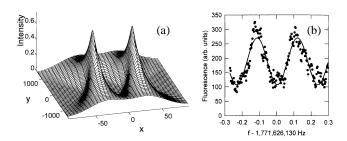
FIG. 15. Light-sheet trap used for rf spectroscopy. (a) Laser intensity produced in a horizontal plane  $30\,\mu\mathrm{m}$  above the intersection of the two focused sheets of light. The x,y dimensions are in microns, and the intensity is normalized to the peak laser intensity. (b) The central Ramsey fringes observed for rf-induced hyperfine transitions for a measurement time of 4 s. From Davidson et al. (1995).
