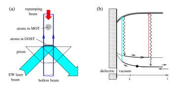
FIG. 20. (a) Schematic of the gravito-optical surface trap (GOST). (b) Illustration of the evanescent-wave cooling cycle. The dot indicates an atom approaching the dielectric surface in the lower hyperfine state, scatters an EW photon, leaves the EW in the upper, less repulsive ground state, and is finally pumped back into the lower state.
