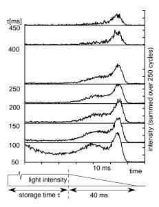
FIG. 13. Time-of-flight spectra of metastable argon atoms trapped in the nodes of a three-dimensional far-off resonance optical lattice. The spectra were taken after various storage times  $\tau$ . Atoms were released from the trap by slowly ramping down the trapping light intensity. Higher-energetic bound states arrive first, deeper confined states later. After long storage times, only atoms in the lowest bound state are found. From Müller-Seydlitz et al. (1998).
