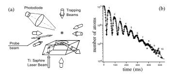
FIG. 19. Observation of atoms bouncing in a gravito-optical cavity. (a) Experimental set-up, and (b) number of atoms detected in the probe beam for different times after their release (points). The solid curve is the result of a corresponding Monte-Carlo simulation. Adapted from Aminoff et al. (1993).
