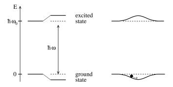
FIG. 1. Light shifts for a two-level atom. Left-hand side, red-detuned light ( $\Delta < 0$ ) shifts the ground state down and the excited state up by same amounts. Right-hand side, a spatially inhomogeneous field like a Gaussian laser beam produces a ground-state potential well, in which an atom can be trapped.
