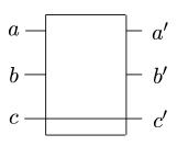
Construct AND, NOT, and OR gates using circuits with just Fredkin gates.
