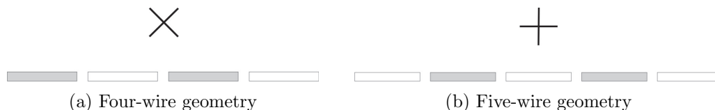
Figure 1.6: Possible configurations for surface-electrode trap. Modified from (14)
