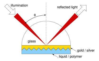
Figure 2: SPR setup for a grating
