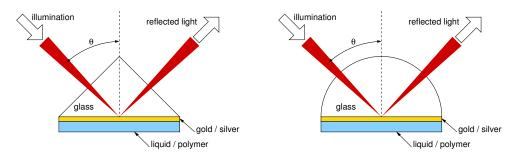
Figure 1: (left) SPR setup using a  $90^{\circ}$  prism. (right) SPR setup using a cylindrical prism.
