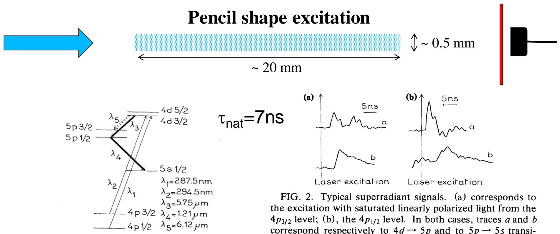
FIG. 2. Typical superradiant signals. (a) corresponds to the excitation with saturated linearly polarized light from the  $4p_{3/2}$  level; (b), the  $4p_{1/2}$  level. In both cases, traces *a* and *b* correspond respectively to  $4d \rightarrow 5p$  and to  $5p \rightarrow 5s$  transitions. The visible oscillations of the signals are most likely due to the hyperfine structure of the  $5p_{1/2}$  level.
