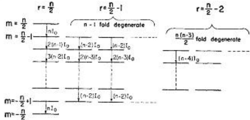
FIG. 1. Energy level diagram of an  $n$ -molecule gas, each molecule having 2 nondegenerate energy levels. Spontaneous radiation rates are indicated.  $E_m = m E_r$ .
