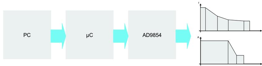
Figure A.3.: Basic idea for generating the frequency and amplitude ramps: Amplitude and frequency ramps are programmed on a PC and stored on a microcontroller ( $\mu C$ ). Upon request they are then sent to the AD9854, which generates the corresponding RF signal.
