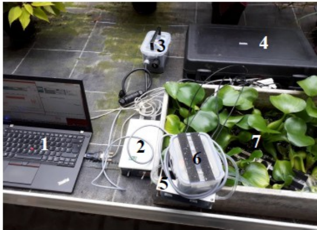
Figure 02 Photograph of the measurement setup, 1: data logger; 2 control unit; 3: energy supply; 4: measuring case with fiber optic meters; 5: sensor unit; 6: pump unit; 7: cuvette with carrier plate
