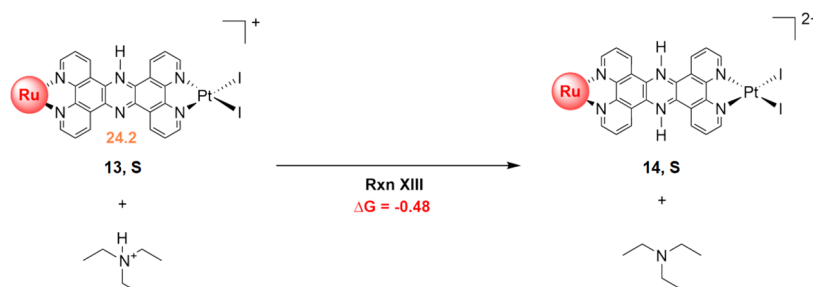
Scheme 3. Possible Reaction Mechanism for the Double Protonation of the Bridging Ligand
