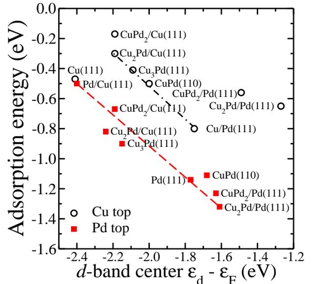
FIG. 5: CO adsorption energies at the top Cu and Pd sites as a function of the  $d$ -band center at various PdCu alloy surfaces. The lines are plotted as a guide to the eye.
