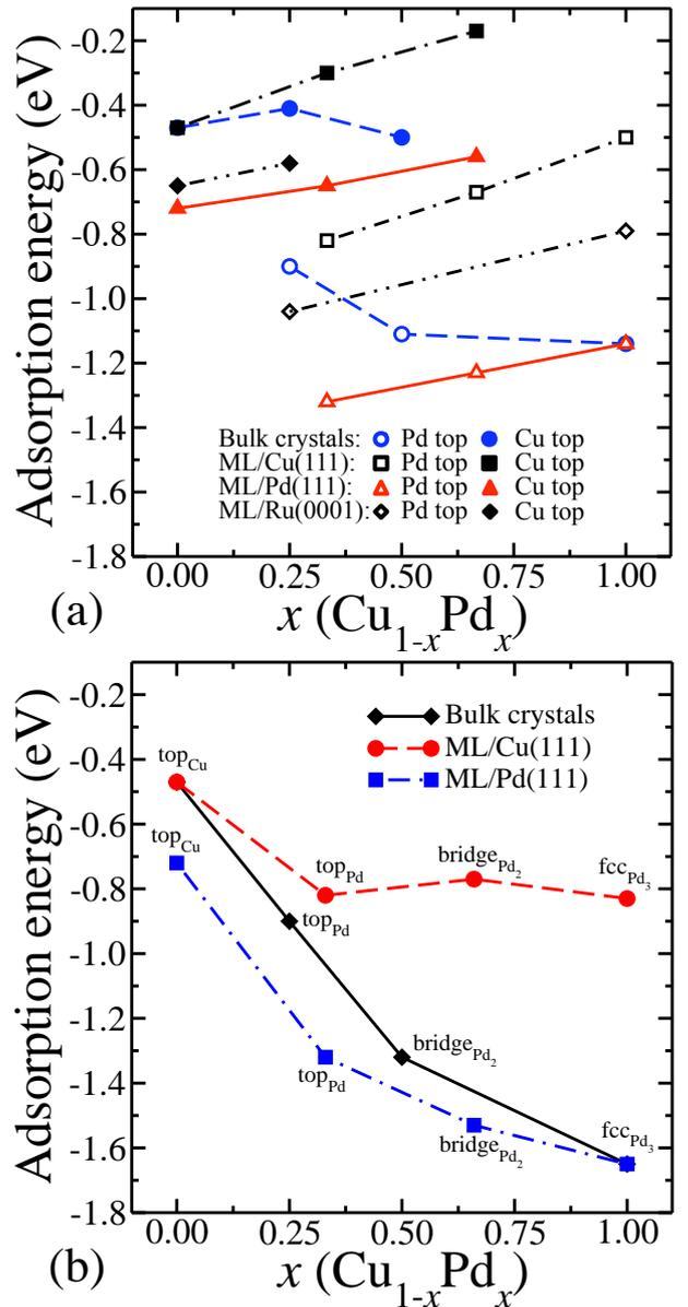
FIG. 4: CO adsorption energies as a function of the Pd concentration  $x$  on various alloy surfaces at the top sites of Pd and Cu (a) and at the most favorable sites (b).
