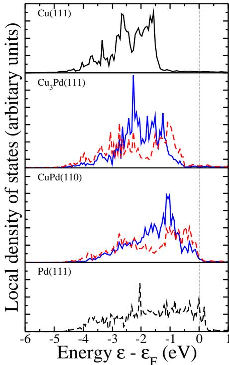
FIG. 2: Local  $d$ -band density of states of  $\text{Cu}_3\text{Pd}(111)$  and  $\text{CuPd}(110)$  bulk alloy surfaces compared to clean  $\text{Cu}(111)$  and  $\text{Pd}(111)$ . The Cu  $d$ -states are represented by solid lines, the Pd states by dashed-lines.
