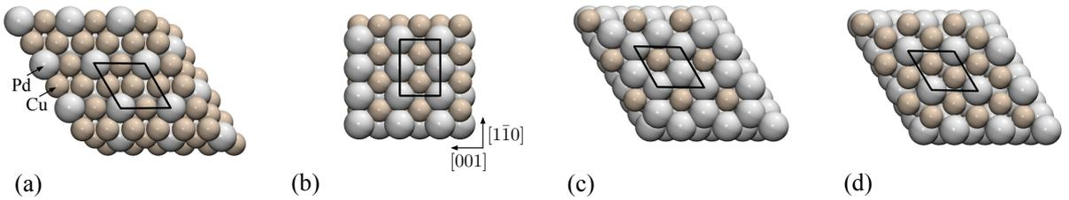
FIG. 1: Illustration of the bimetallic surface structures addressed in this study including the used surface unit cells for CO adsorption. a)  $\text{Cu}_3\text{Pd}(111)$  b)  $\text{CuPd}(110)$ , c)  $\text{CuPd}_2/\text{Pd}(111)$ , d)  $\text{Cu}_2\text{Pd}/\text{Pd}(111)$ .
