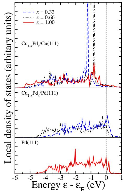
FIG. 3: The Pd d-band local density of states of monolayer alloys on Cu(111) (upper panel) and on Pd(111) (middle panel) for various Pd concentrations compared with the LDOS of pure Pd(111) (lower panel). The Pd d-band width increases with increasing Pd content. On Cu, the Pd bands are shifted to lower energies caused by the 8% suppression.
