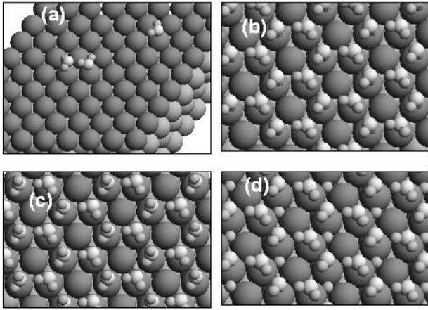
FIG. 1: Water structures on a Pd/Au(111) overlayer. a) equilibrium structure of the water monomer and dimer, b) H-down bilayer, c) H-up bilayer, d) half-dissociated water bilayer.
