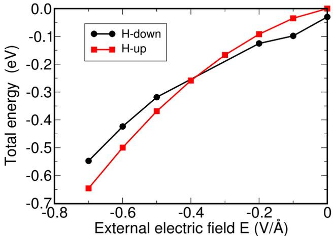
FIG. 5: Change of the total energy of the H-down and H-up water bilayers as a function of the external electric field. The energy zero corresponds to the H-up structure without any external electric field.
