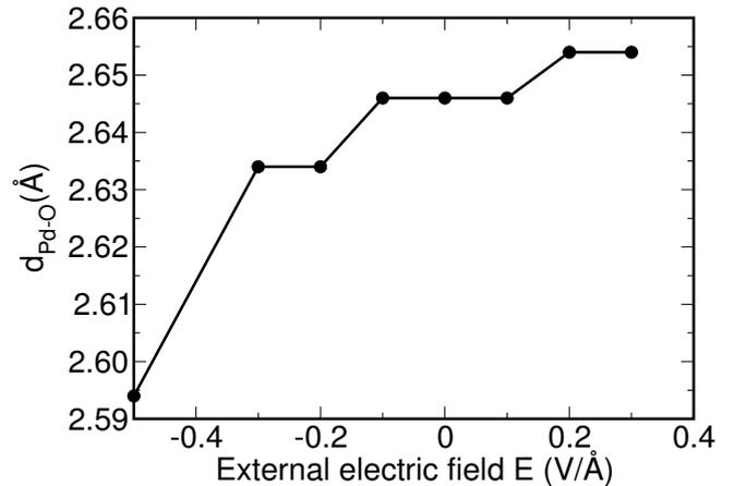
FIG. 4: Distance of the oxygen atom  $d_{\text{Pd-O}}$  of the water molecule from the surface in Å as a function of the external electric field.
