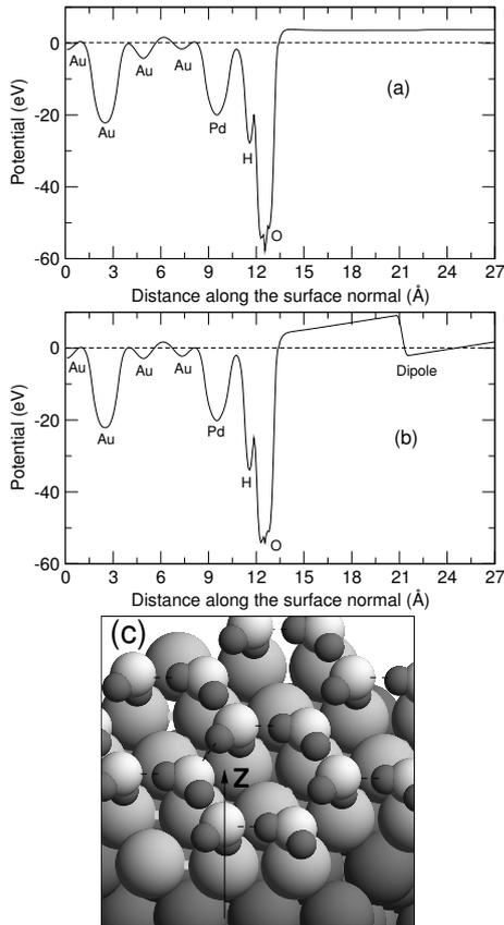
FIG. 3: Effective potential along the surface normal  $z$  which passes through the water molecule for (a) zero external field, (b)  $E = -0.7 \text{ V/Å}$ , (c) illustrates the location of the  $z$  axis.
