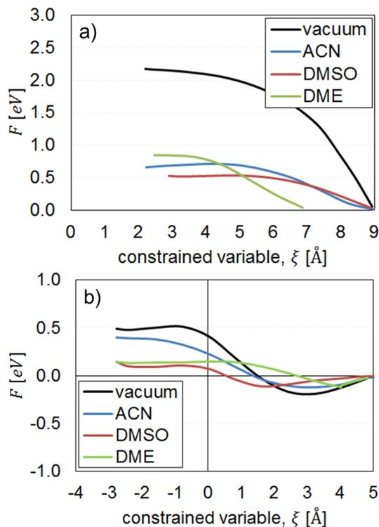
Figure 5: Reaction energy barriers obtained from the Blue Moon method of AIMD simulations for a) (Association)  $\text{Li} + \text{O}_2 \rightarrow \text{LiO}_2$  and b) (Disproportionation)  $2(\text{LiO}_2) \rightarrow \text{Li}_2\text{O}_2 + \text{O}_2$  in vacuum and 1 M of each of ACN, DMSO and DME electrolytes.
