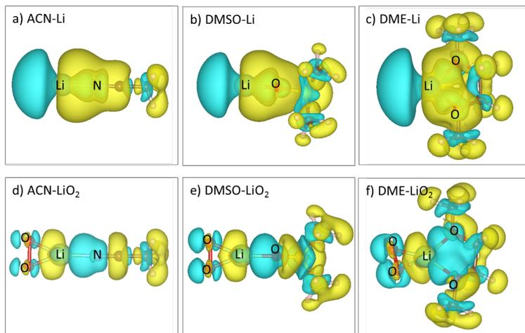
Figure 1: Charge density difference  $\Delta\rho$  upon the interaction of Li with a) ACN, b) DMSO and c) DME molecules, and  $\text{LiO}_2$  with d) ACN, e) DMSO and f) DME molecules, as obtained from DFT calculations using Eq. 2. Cyan and yellow regions correspond to electron accumulation and depletion, respectively. The isosurface levels are  $\pm 0.005 \text{ eV \AA}^{-3}$ .
