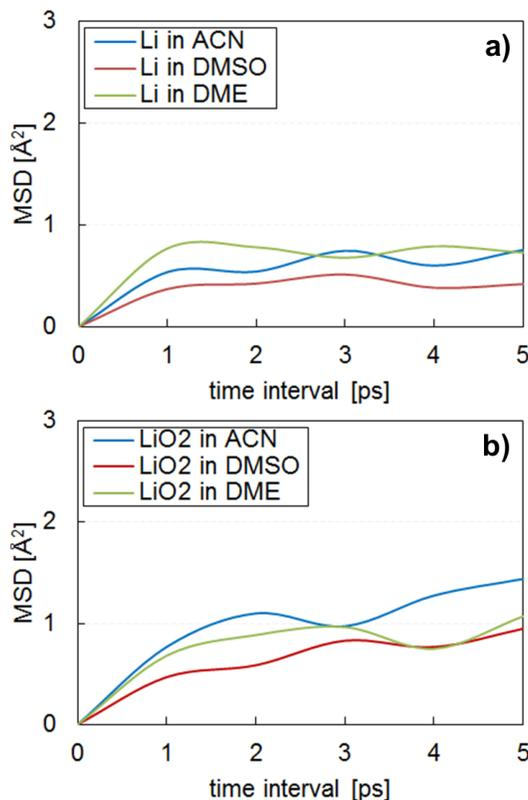
Figure 4: Mean square displacement (MSD) obtained from AIMD simulations of a) Li and b) LiO<sub>2</sub> in 1 M of each of ACN, DMSO and DME electrolytes.
