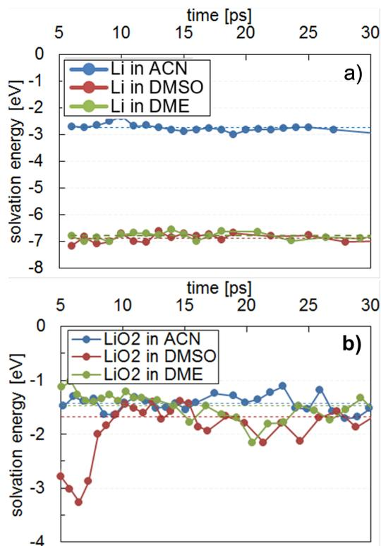
Figure 3: Solvation energies obtained from AIMD simulations of a) Li and b) LiO<sub>2</sub> in 1 M of each of ACN, DMSO and DME electrolytes.
