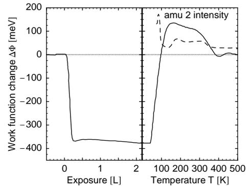
FIG. 3: Hydrogen-induced work function change  $\Delta\Phi$ . a) Dependence of  $\Delta\Phi$  on  $\text{H}_2$  exposure for adsorption at 50 K. b) Dependence of  $\Delta\Phi$  on the surface temperature after saturation of the Pd(210) with molecular hydrogen. The  $\text{H}_2$  TPD spectrum (dashed line, arbitrary units) is also plotted.
