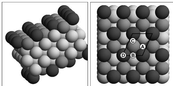
FIG. 1: Side and top view of the (210) surface. In the right panel the surface unit cell plus the three atomic adsorption sites A, B, and C are included. The site D corresponds to the molecular adsorption site.
