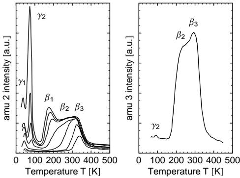
FIG. 2: Thermal desorption spectra. a) Series of  $\text{H}_2$  TPD spectra for different exposures between 0.02 L and 0.2 L at a temperature of 50 K. b) Mass 3 (HD) TPD spectrum after a mixed  $\text{H}_2/\text{D}_2$  exposure at 50 K.
