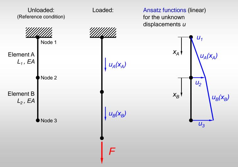
The unknown displacement function of the entire rod is described with a series of simple (linear) **ansatz functions** (see figure). This is the **basic concept** of FEM.
