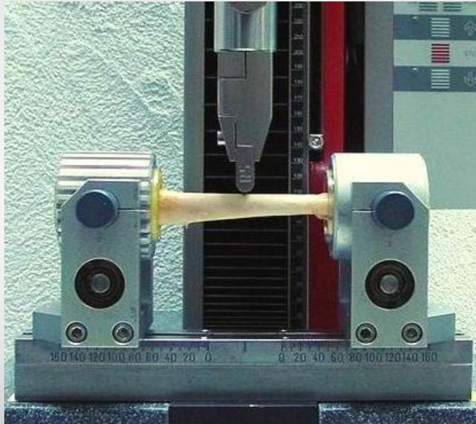
3-Point Bending of a bone specimen
