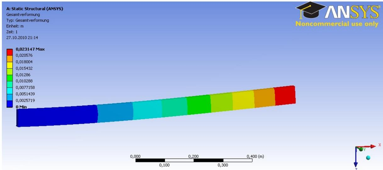
Figure 17: Deformed shape of the beam resulting from corrected force.
