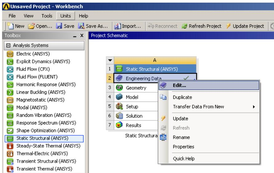
Figure 8: Assignment of the engineering data
