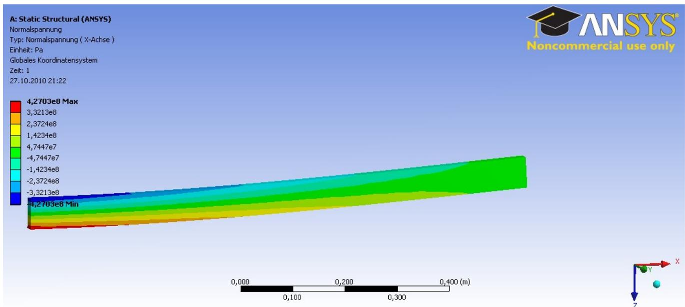
Figure 19: Contour plot of x-component of stress.
