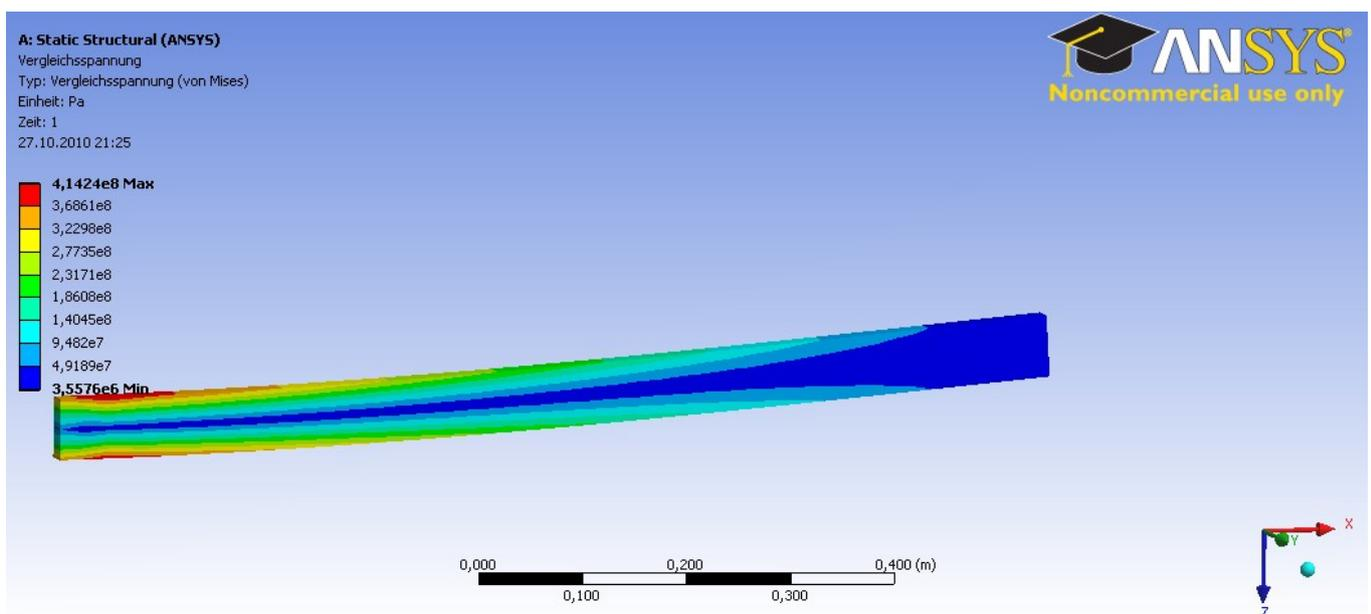
Figure 20: Contour plot of Von-Mises equivalent stress.
