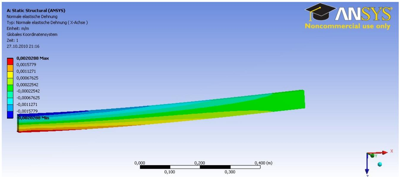
Figure 18: Contour plot of x-component of total strain.
