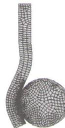
This exercise has two purposes: (1) to demonstrate how to apply a simple initial condition, namely uniform velocity, on a body, and (2) to show a limitation of <Transient Structural> analysis system for impact simulations, and to build a learning motivation for <Explicit Dynamics> (Chapter 15).
