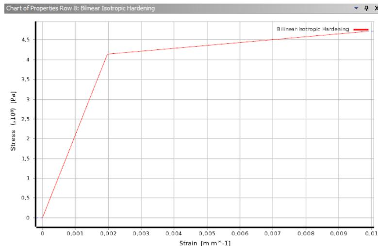
FIGURE 2: STRESS-STRAIN CURVE FOR OUR ELASTO-PLASTIC MATERIAL
