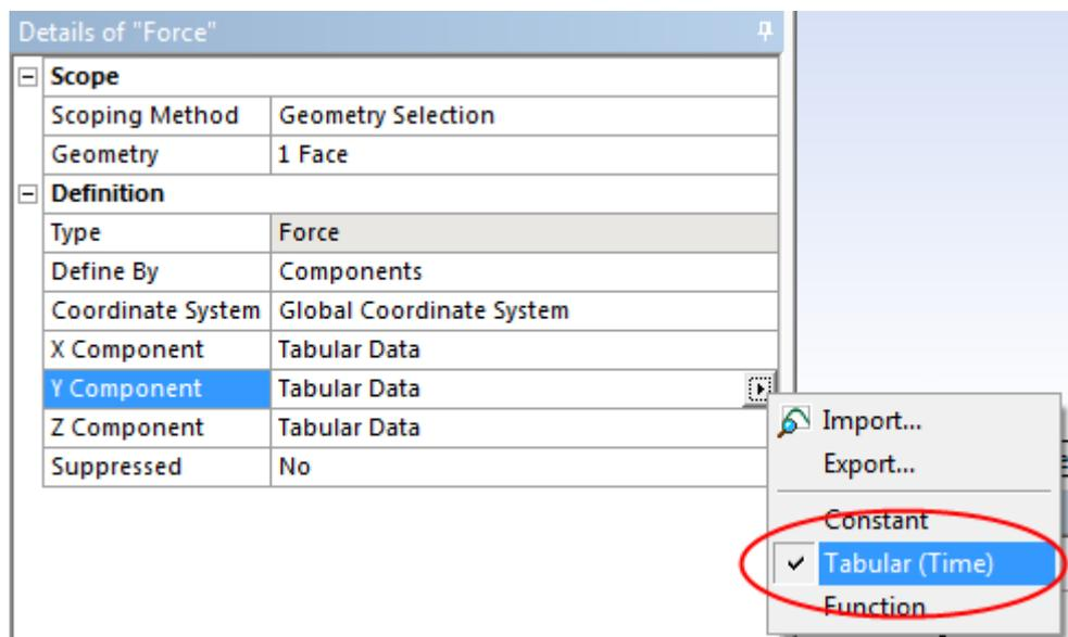
FIGURE 3: USING TABULAR DATA FOR THE FORCE COMPONENTS
