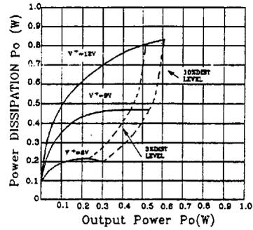
**Power Dissipation vs. Output Power (RL=16Ω)**
